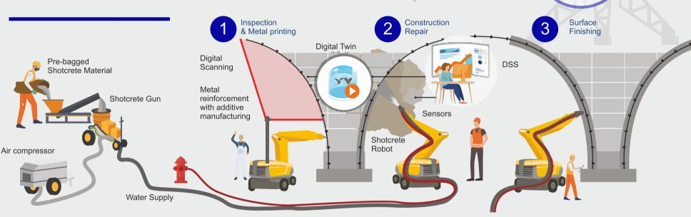
RoBétArmé aims toward a step-change in Construction 4.0 by automating particularly laborious construction tasks in all phases of shotcrete application.
