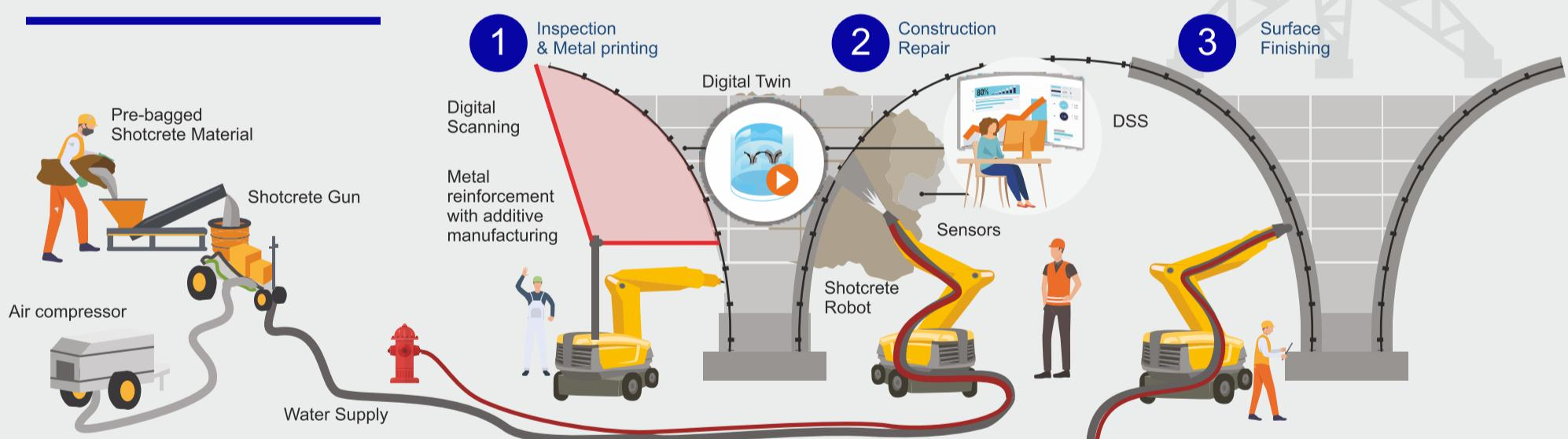
RoBétArmé aims toward a step-change in **Construction 4.0** by automating particularly laborious construction tasks in all phases of shotcrete application.
